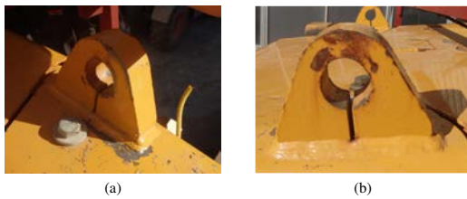
Fig. 14. Results of the real structural test show that the actual deformations differ from the results provided by the non-linear FE-simulations.
