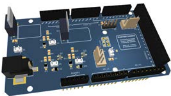
Fig. 7. Extension board for MCU Arduino Mega 2560
