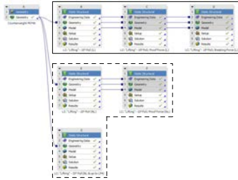
Fig. 5. Ansys Workbench project for one component and load case.
