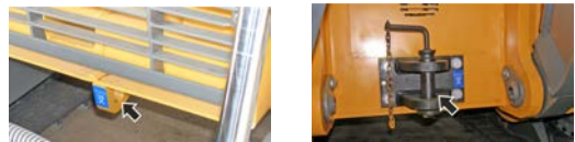
Fig. 1. Example of an eyehook serving as a front lashing point (a) and as a rear lashing & retrieval point (b) of a crawler tractor, both taken from [4].
