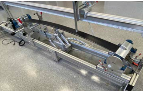
Fig. 7. Bending test: A ski in the deformed measurement configuration within the STB.
