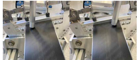
Fig. 13. Torsion test: Cross-section of the ski is rotated around its centre line. Two traces are recorded during the measurement to recalculate the torsion angle \theta .
